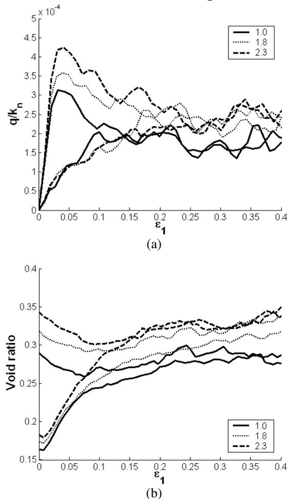
Fig. 1. Evolution of (a) the deviator stress (b) void ratio during the biaxial test for different ratios of particle elongation.
