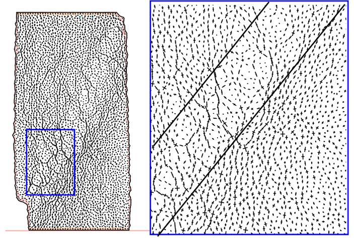
Figure 2: Principal stress directions of the individual grains after failure ( $\epsilon_1 = 0.07$ ). The confining pressure is  $p_0 = 160 \text{ kPa}$ .
