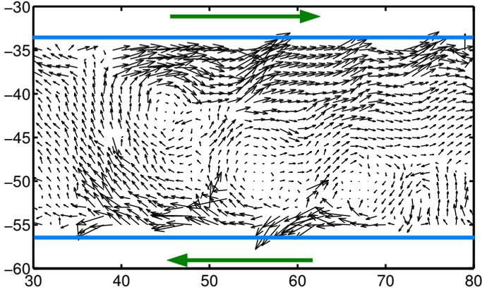
Figure 3: Displacement field in the shear cell
