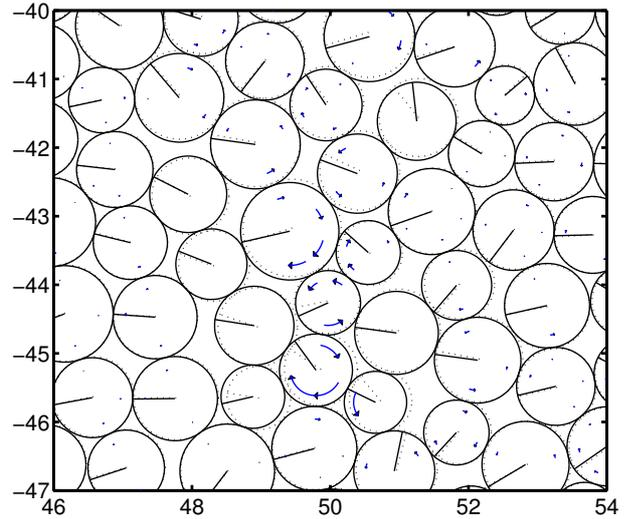
Figure 5: Displacement at the contacts.
