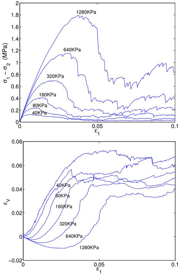
Figure 1: Deviatoric stress and volumetric strain versus axial strain for different confining pressures.
